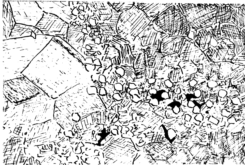
Fig. 5. Skegby Quarry x 30 Coarse dolomitic limestone with band of finer dolomite and detrital quartz. Interstitial galena.
